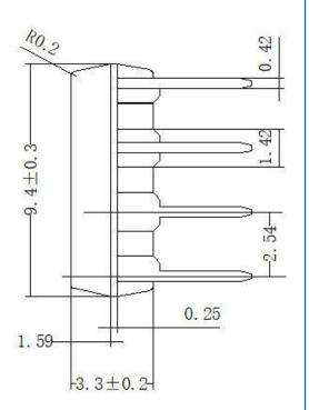
Note: No tolerance is marked as ±0.05mm.
