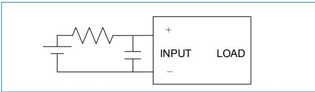
D. Recommended to use the circuit, the output peak voltage may cause SSR misoperation, so please add R/C circuit or varistor to absorb the peak voltage at the output end, see the following figure:
